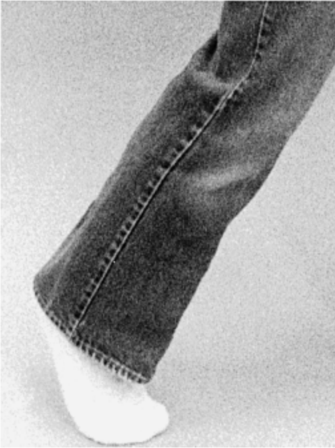
FIG. 1—Pucker or “ridge-and-valley” pattern along seam of blue jeans resembles a “barcode.”
